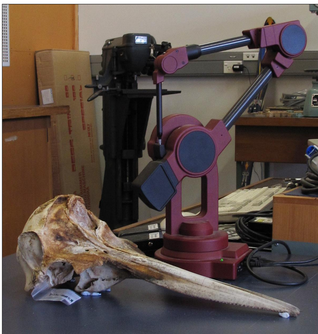
Plate 2.4. Setup for the digitization process of cranial landmark acquisition on Delphinus sp. skull from New Zealand waters with a microscribe.
